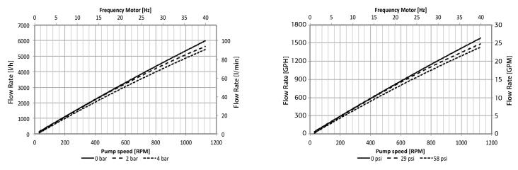
Depending on the selected motor/frequency drive combination, the motor frequency and the resulting pump speed might differ.
