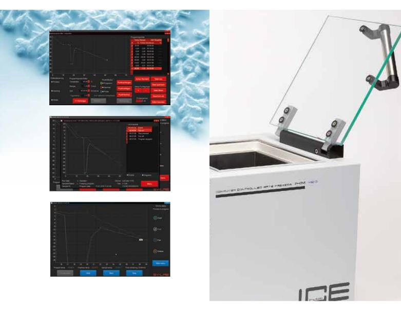
permitting unobstructed views of the items being frozen across a wide range of temperatures. When opening during the freezing process the operation is interrupted on safety grounds. Alongside the sensor for the chamber temperature there is also a sensor for the sample temperature.
